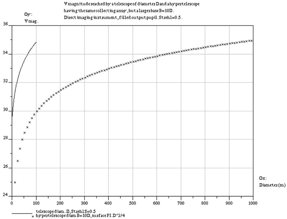
**Figure 5.** V magnitude ( $S/N = 5$  in 1000s, Strehl=50%) reached by a telescope of diameter  $D$  (solid curve at left) and a hypertelescope (curve at right) having the *same collecting area*, but a *larger baseline*  $B = 10 \times D$ . For example, the 50m ELT and the 500m baseline hypertelescope will reach the same limit magnitude ( $V \approx 33.5$ ), providing both have the same collecting area.
