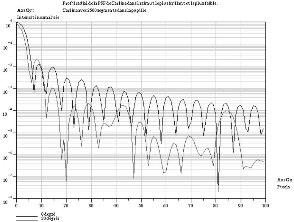
**Figure 4.** Cuts in the Carlina PSF in the brightest (above) and darkest (below) radial directions. Each bump (upper curve for example) is  $\approx \lambda/B$  wide.
