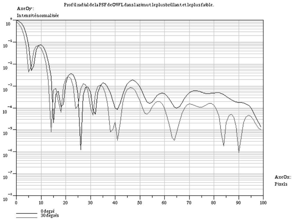
**Figure 3.** Cuts in the OWL PSF in the brightest (above) and darkest (below) radial directions. Each bump (upper curve for example) is  $\approx \lambda/B$  wide.
