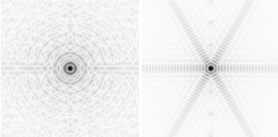
**Figure 2.** PSF for ELT OWL<sup>2</sup> (left) and a hypertelescope with 2500 segments, Carlina<sup>8</sup> (right). Intensity is represented with the same log scale on both figures. The log scale intensifies the speckles around the central core. The exact pupil shapes are taken into account (including the 4mm gap between OWL segments).
