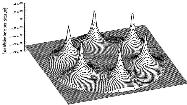
Fig. 2. Estimated extra deflection caused by shear forces, as computed for the ESO NTT 3.6-m primary mirror (Table 1) on a hypothetical six-point support with sixfold symmetry. This simple support, instead of the real 78-point one, was chosen for clarity.
