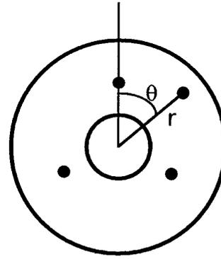
Fig. 1. Top view of a mirror with a central hole. In this example, four discrete axial forces are applied to the mirror. Three of them are arranged with threefold symmetry.
