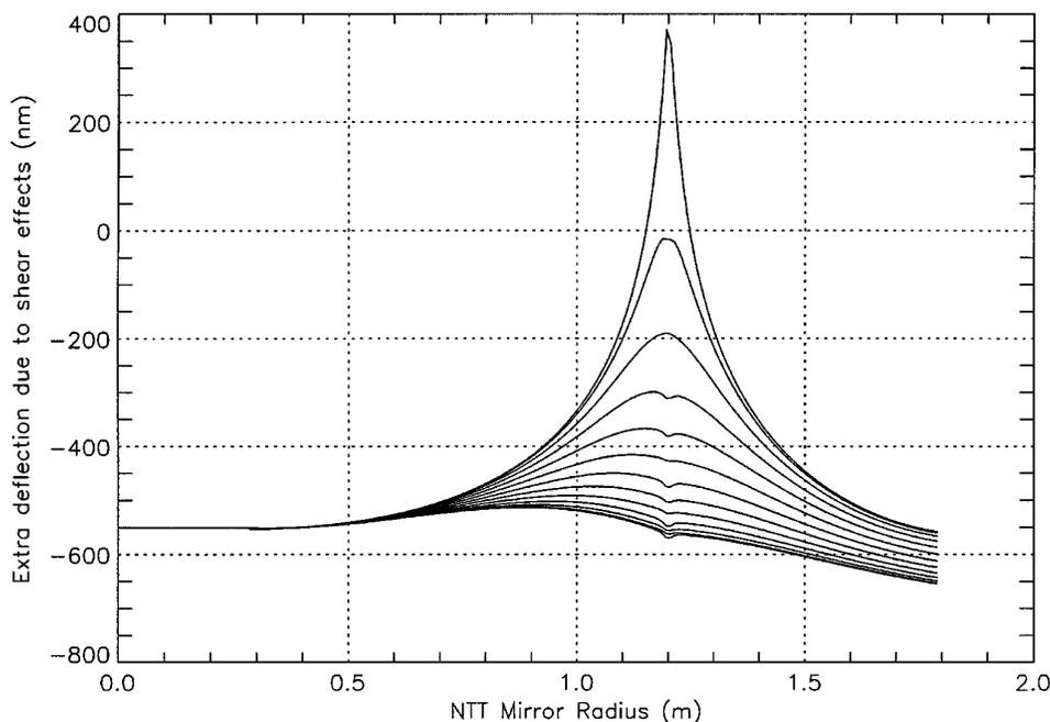
Fig. 3. Radial shear deflections, equally angularly spaced, for azimuth on the mirror going from a radius with a supporting point to a radius between two supporting points. The artifact along the supporting radius (1.2 m) is visible. The same six-point support as in Fig. 2 is shown.
