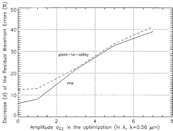
Fig. 5. NTT primary-mirror active support: computed decrease  $d$  of the residual wave-front error obtained with optimized active supports with respect to the residual wave-front error obtained by the current ESO NTT active support. The topologies are optimized only over the clear aperture, from the internal stop to the outer edge. The improvement in the wave front is calculated with respect to the performances measured over the same clear aperture for the current support.
