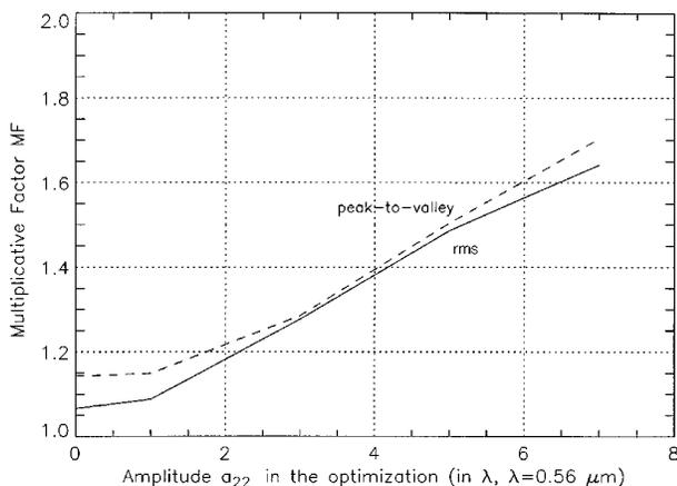
Fig. 6. NTT primary-mirror active support: expected multiplicative factor  $MF$  applied to the correction range from the current ESO NTT active support for the case of astigmatic correction.
