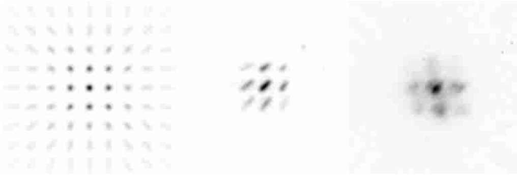
Fig. 6. Numerical simulation of PSF for the instrument (left) with the pupil densifier removed (Fizeau mode), in densified-pupil mode on a dispersed order (centre) and the star \alpha Gem (right). Comparing the star image to the numerically simulated PSF we deduced that pointing errors positioned the object outside the field of view of the interferometer. The result is a dispersed image of the double star
