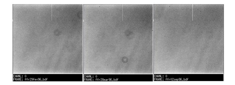
This illustrates the pitfalls when using flat-fields taken at other times: the dust specks on the dewar window have moved !
