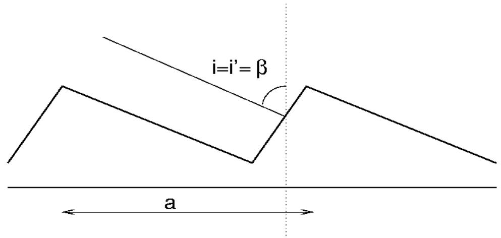
Echelle grating: small incidence angle: allows to work in a large order: increase of spectral resolution
