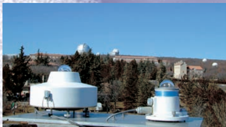
In the foreground are visible two pyranometers which measure sunlight continuously, both in the entire spectrum and in the UV, for the study of the Earth's atmosphere.
