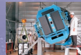
The VIMOS spectrograph undergoing integration at OHP. It is now operating at one of the European Southern Observatory's VLT telescopes in Chile.
